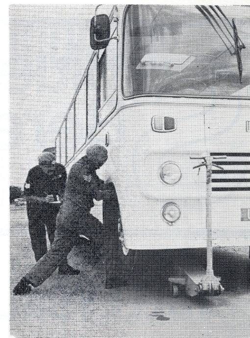
Sgt John Wilkinson and Sgt Alan Clifton carry out an inspection of a UN bus, in this case wheel bearings.
