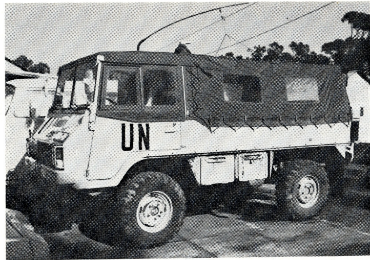
Pinzgauer (2-Achser): Payload 1000 kg; own weight 2050 kg; highest speed 105 km/h; 87 PS; hill-climbing-ability until the limit of adhesion.
